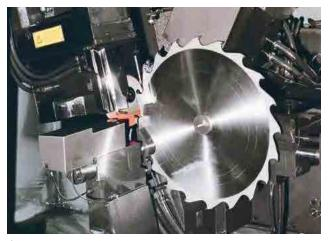
Grinding and tensioning the blades.
