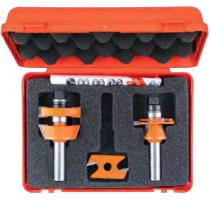
These new bit sets are excellent for producing adjustable tongue and groove joints with a bevel, in order to eliminate the panel rattle that may come up with the production of standards cabinets. Cut precise grooves into your plywood veneered panels and make perfect rattle-free fits. To be used on table-mounted routers. Avoid using these bits in hand-held power tools.
