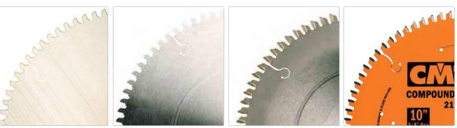
Laser cutting The steel plate of the blade is laser cut, NEVER die cut, from superior strength steel. This way of cutting steel is not only extremely precise but it makes it possible to cut harder strengths of steel and does not stress the plate while cutting, so the resulting blade is flat and true and more resistant to warping.
