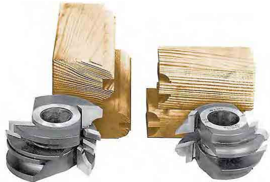
1 3 / 8 " Interior Profile, using one spacer & the 1/4" groover.
